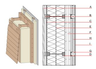
Note: Attention: REI 90 (from inside) in Germany possible with 2x12,5mmgypsum plaster board type DF/gypsum fibre board
