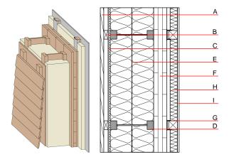
Note: Attention: REI 90 (from inside) in Germany possible with 2x12,5mm gypsum plaster board type DF/gypsum fibre board
