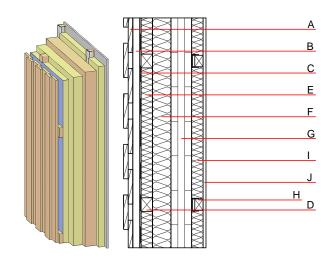
Note: When using cross laminated timber: Variation 00-03: d  $\geq$  94,0; at least 3-layers, top layer at least 30mm; variation 04: d  $\geq$  78,0; at least 3-layers, top layer at least 25mm
