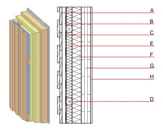
Note: When using cross laminated timber: Variation 02-03: d  $\geq$  94,0; at least 3-layers, top layer at least 30mm; variation 00-01: d  $\geq$  78,0; at least 3-layers, top layer at least 25mm
