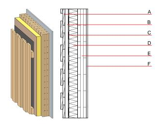
Note: When using cross laminated timber: Variation 00-03: d ≥ 78,0; at least 3-layers, top layer at least 25mm; variation 04: d  $\geq$  94,0; at least 3-layers, top layer at least 30mm
