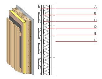
Note: When using cross laminated timber: Variation 00-03: d ≥ 78,0; at least 3-layers, top layer at least 25mm; variation 04: d  $\geq$  94,0; at least 3-layers, top layer at least 30mm D=2x60 mm
