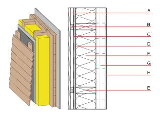
Note: Cross laminated timber: Variation 00-02 and 04-06: at least 3-layers, top layer at least 30mm; variation 03:  $d \ge 85,0$ ; at least 5-layers, top layer at least 17 mm
