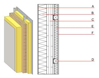
Note: Attention: REI9O (from inside) in Germany possible with 2x12,5mm gypsum plaster board type DF/gypsum fibre board
