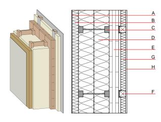
Note: Attention: REI 90 (from inside) in Germany possible with 2x12,5mm gypsum plaster board type DF/gypsum fibre board
