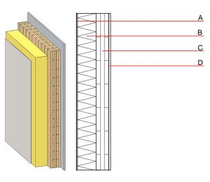
Note: Cross laminated timber: Variation 00-03: d  $\geq$  78,0; at least 3-layers, top layer at least 25 mm; variation 04-07: at least 3-layers, top layer at least 30 mm
