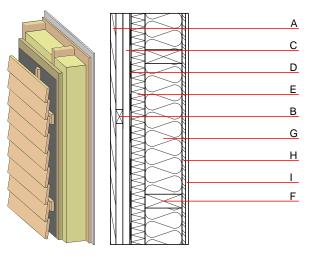
Note: According to OIB-RL 2 (Austria) is for ventilated and insulated facades (from building class 2) an insulation material with minimum Euroclass D required.
