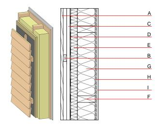
Note: According to OIB-RL 2 (Austria) is for ventilated and insulated facades (from building class 2) an insulation material with minimum Euroclass D required.
