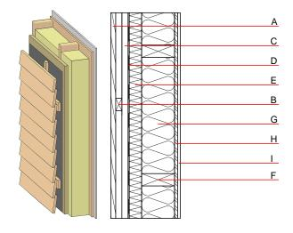
Note: According to OIB-RL 2 (Austria) is for ventilated and insulated facades (from building class 2) an insulation material with minimum Euroclass D
