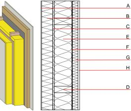
Register of building materials used for this application, cross-section (from outside to inside, dimensions in mm)
