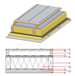
Note: The design of the under-roof construction and of the counterbattens have to be specified according to the roof pitch and the national requirements. J=without insulation
