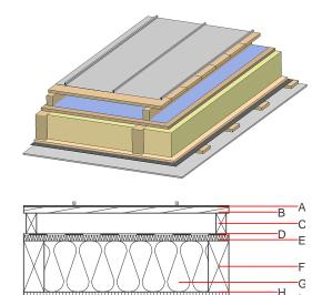
Note: The design of the under-roof construction and of the counterbattens have to be specified according to the roof pitch and the national requirements.
