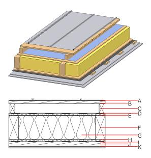
Note: The design of the under-roof construction and of the counterbattens have to be specified according to the roof pitch and the national requirements.
