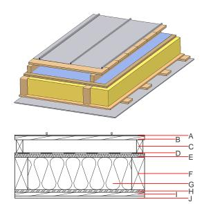
Note: The design of the under-roof construction and of the counterbattens have to be specified according to the roof pitch and the national requirements.
