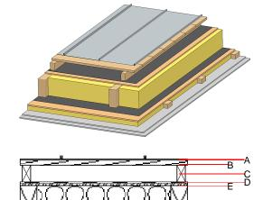
Note: The design of the under-roof construction and of the counterbattens have to be specified according to the roof pitch and the national requirements.
