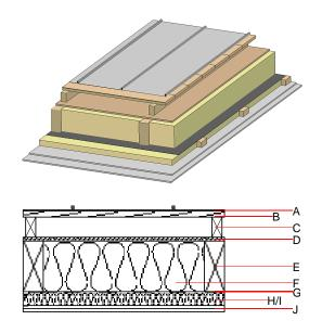
Note: The design of the under-roof construction and of the counterbattens have to be specified according to the roof pitch and the national requirements. I=without insulation
