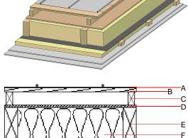
Note: The design of the under-roof construction and of the counterbattens have to be specified according to the roof pitch and the national requirements.
