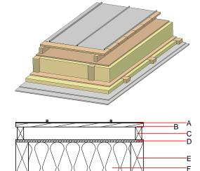
Note: The design of the under-roof construction and of the counterbattens have to be specified according to the roof pitch and the national requirements.
