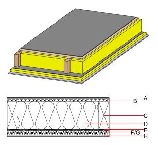
Note: ATTENTION: Regarding protection against moisture an objectrelated proof in terms of paramter like e.g. climate, shading class etc. is required. Therfore a hygrothermic simulation is necessary (e.g.WUFI), a simple Glaser calculation ist not allowed.
