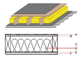
Note: ATTENTION: Regarding protection against moisture an objectrelated proof in terms of paramter like e.g. climate, shading class etc. is required. Therfore a hygrothermic simulation is necessary (e.g.WUFI), a simple Glaser calculation ist not allowed.
