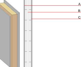
Note: The fire resistance is only valid when wall is used as partition with only one side exposed to fire. Cross laminated timber:
