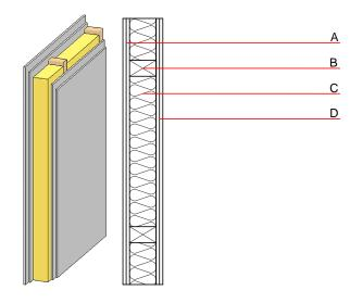
Note: The fire resistance is only valid when wall is used as partition with only one side exposed to fire. (B=60/100); e=625
