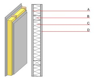
Note: The fire resistance is only valid when wall is used as partition with only one side exposed to fire. (B=60/100); e=400
