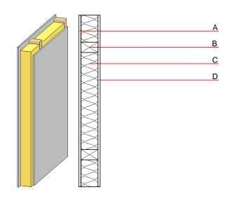
Note: The fire resistance is only valid when wall is used as partition with only one side exposed to fire. (B=60/160); e=625
