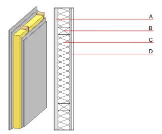
Note: The fire resistance is only valid when wall is used as partition with only one side exposed to fire. (B=60/100); e=625
