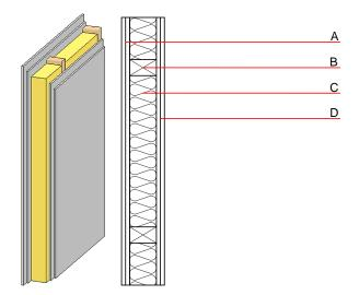
Note: The fire resistance is only valid when wall is used as partition with only one side exposed to fire. (B=60/160); e=400
