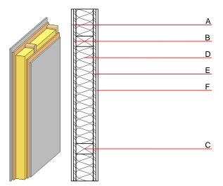
Note: The fire resistance is only valid when wall is used as partition with only one side exposed to fire. (C=60/100); e=400
