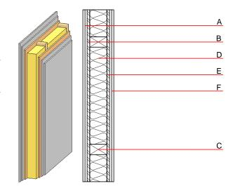
Note: The fire resistance is only valid when wall is used as partition with only one side exposed to fire. (C=60/100); e=625
