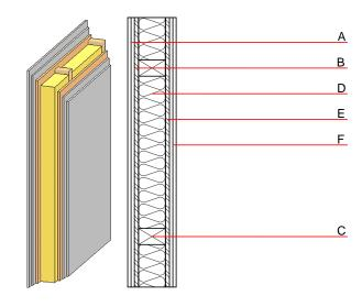
Note: The fire resistance is only valid when wall is used as partition with only one side exposed to fire. (C=60/100); e=625
