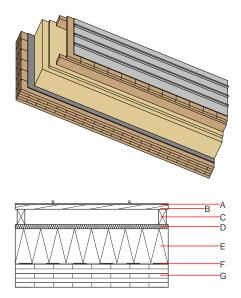
Note: The design of the under-roof construction and of the counterbattens have to be specified according to the roof pitch and the national requirements. Underlay laminated on insulation board
