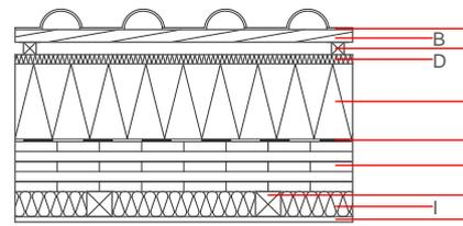
**Note:** The design of the under-roof construction and of the counter-battens have to be specified according to the roof pitch and the national requirements.
