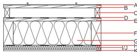
**Note:** The design of the under-roof construction and of the counter-battens have to be specified according to the roof pitch and the national requirements.
