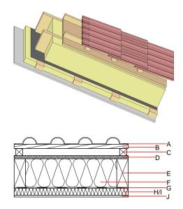
Note: The design of the under-roof construction and of the counterbattens have to be specified according to the roof pitch and the national requirements.
