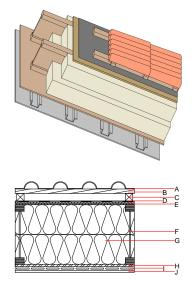
Note: The design of the under-roof construction and of the counterbattens have to be specified according to the roof pitch and the national requirements.
