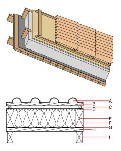
Note: The design of the under-roof construction and of the counterbattens have to be specified according to the roof pitch and the national requirements. Depending on the requirements (eg increased rainproof under-roof), an additional underlay is required.
