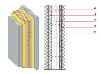
Note: Attention: Composite component (A + wood wool board + DF) selfsupporting as wall covering. Cross laminated timer: thickness ≥ 125mm; 5-ply at least, surface layer at least 27,5mm
